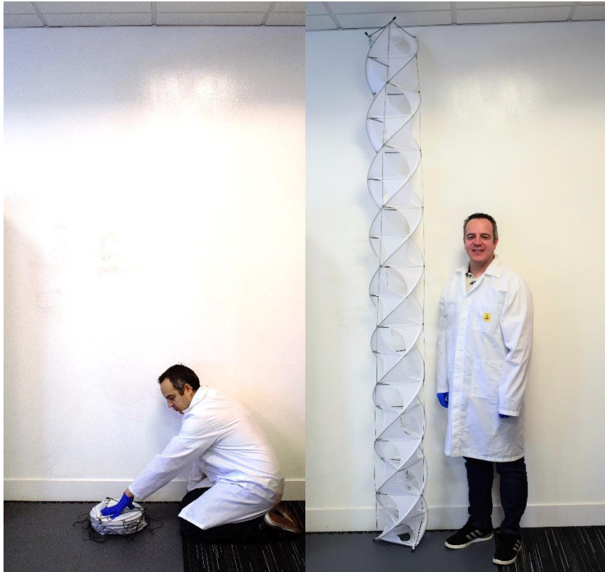
Figure 1: Breadboard prototype of the origami-inspired deployable VHF antenna, stowed (left) and deployed (right).
